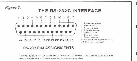
prepared to transmit data. This signal is generated in response to Request to Send. This line may be connected directly to its own Request to Send Line when connecting peripherals.
